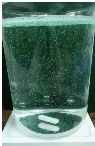
Figure 10. Image of a beaker containing wastewater analogue before the EC process.
